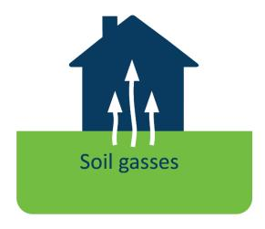
Air moves up and out of buildings, which draws in soil gases, including radon.
