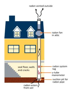
A radon mitigation system added to an existing house usually involves a PVC pipe placed through the house, starting under the slab, sump hole, or drain tile (typically on suction point is sufficient). Radon gas is drawn out of the soil with a fan in the attic and expelled through the roof.
